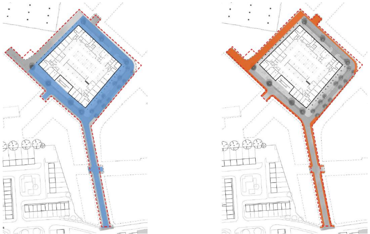
Image 6: Permanent works (left) and temporary works (right) for access
